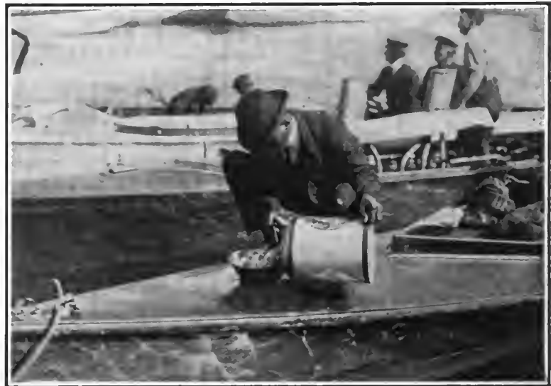
FILLING HIDDEN GASOLINE TANK IN BOW OF AUTO BOAT. AT PALM BEACH.
